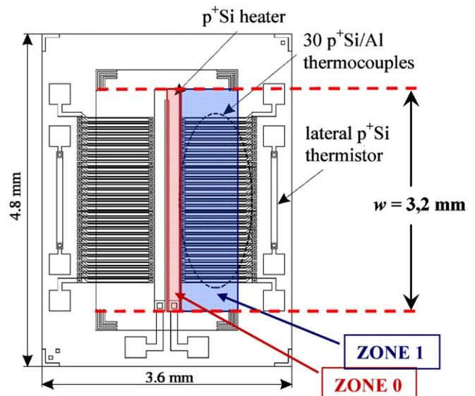
Fig. 2. Partition of sensor in zones 0 and 1, membrane area of interest is marked with dashed lines.
