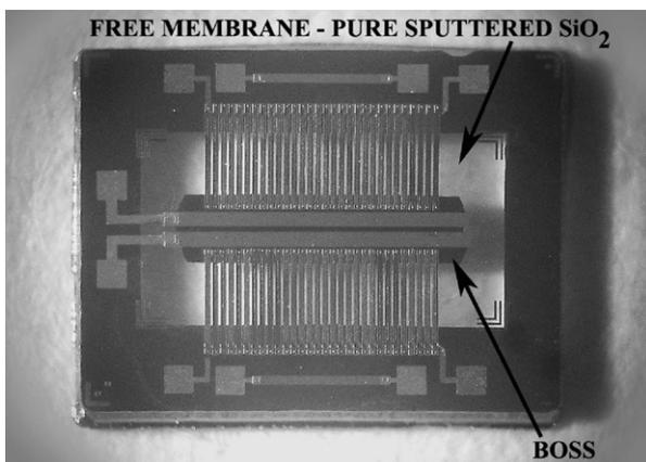
Fig. 1. Thermal sensor with “boss” structure,  $NiCr$  heater and  $NiCr/Au$  thermocouples after complete release of oxide membrane using bulk micromachining.
