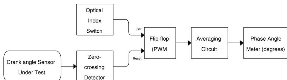
Fig. 2. Test fixture block diagram.
