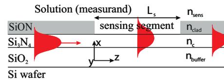
**Fig. 2.** Longitudinal cross-section of the considered slab structure of an SWG sensor consisting of three segments.
