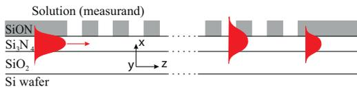
**Fig. 1.** Schematic longitudinal cross-section of a periodic SWG sensor containing about 2000 periods of length 20  $\mu\text{m}$ .
