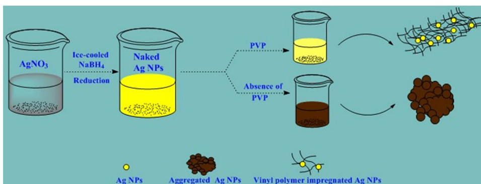
Fig. 1. Schematic diagram on the formation of silver nanoparticles protected/unprotected by vinyl polymer.
