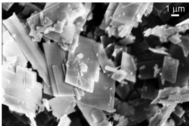
**Fig. 1.** Scanning electron microscopy image of ZrPOF-DEA showing the platelike morphology.
