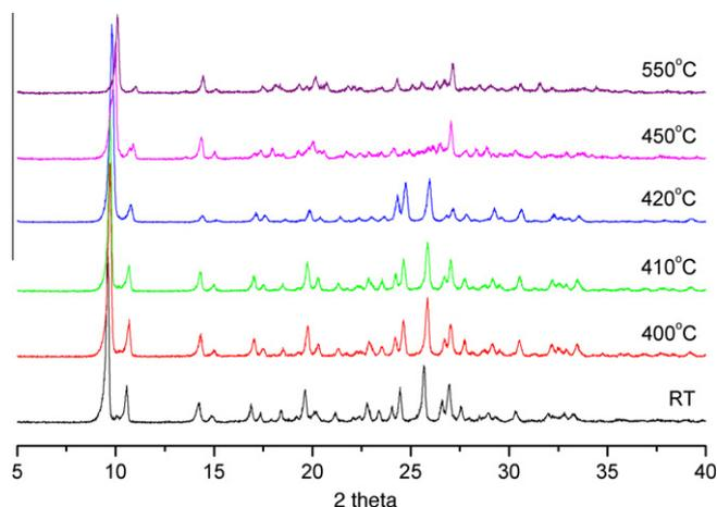
**Fig. 2.** X-ray powder diffraction patterns of ZrPOF-DEA taken after treatment at the temperature indicated for 5 h.
