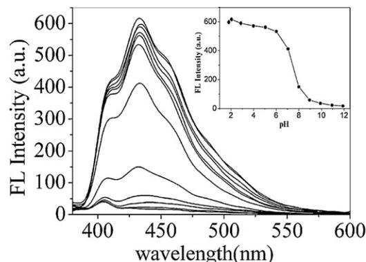
**Fig. 1.** Effect of pH on the fluorescence spectra of BHIA.  $C_{\text{BHIA}} = 8.0 \times 10^{-6} \text{ mol L}^{-1}$ . Inset: fluorescence intensities of BHIA at different pH values.
