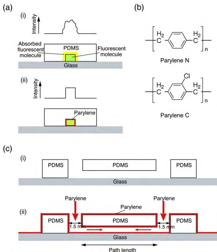
**Fig. 1.** (a) Schematic illustrations of parylene effect in PDMS channels. Fluorescent molecules absorbed in PDMS make channel-crossing line profiles quantitatively poor (i), but parylenes deposited in PDMS channels prevent the absorption (ii). (b) Chemical structures of parylene N and C. (c) Side-view illustrations of PDMS channels without (i) and with a parylene-coat (ii).
