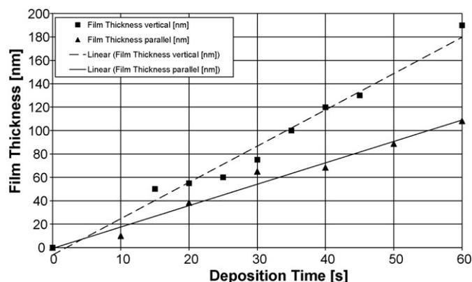
Fig. 2. Film thickness vs. deposition time for perpendicular and parallel atomized spray flow.
