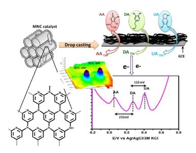
Mesoporous nitrogen rich carbonaceous (MNC) materials have been synthesized at two different temperatures of 600 and 800 °C and explored for simultaneous determination of ascorbic acid (AA), dopamine (DA) and uric acid (UA). The electrocatalytic activity of these materials for the oxidation of analyte molecules was examined by means of redox-competition mode of scanning electrochemical microscopy (SECM), voltammetric, chronoamperometric and rotating disc electrode (RDE) measurements.
