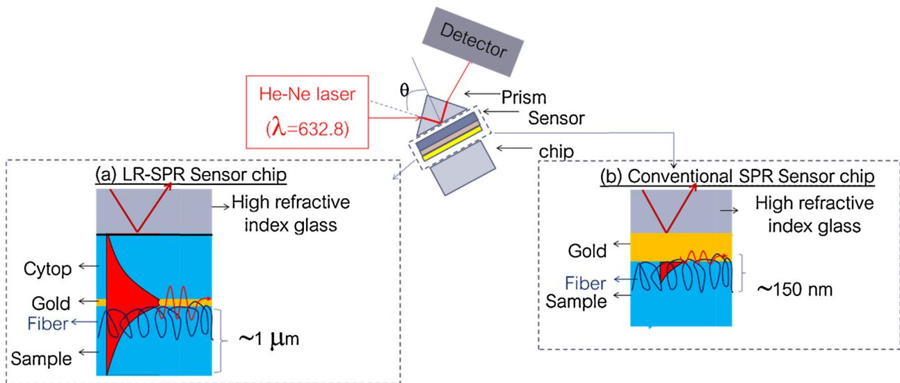
Fig. 1. Schematic of the instrument setup and sensor chip/prism for (a) LR-SPR and (b) conventional SPR at the gold-water interface.
