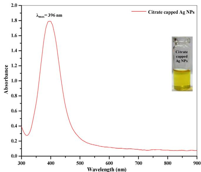
Fig. 1. UV–visible spectrum of citrate-capped Ag NPs. Inset picture show citrate-capped Ag NPs.
