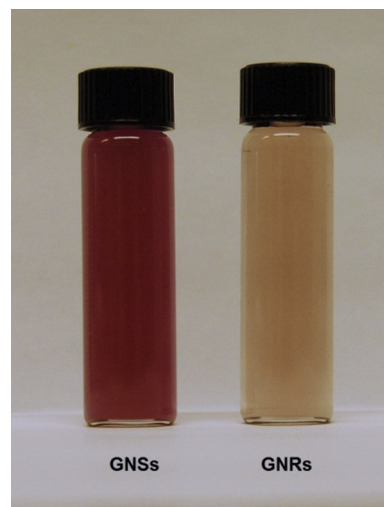
Fig. 1. Illustration of 60 nm GNS solution (left) and GNR solution with an aspect ratio of 4.1 (right).
