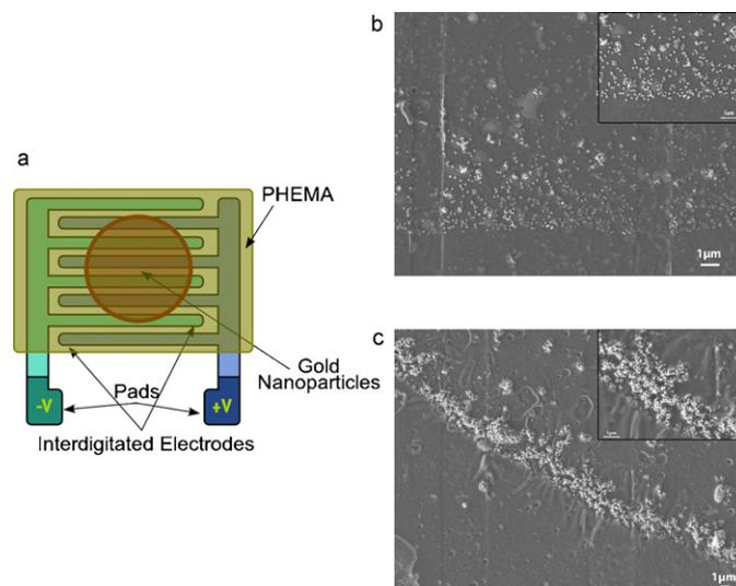
**Fig. 2.** FESEM images of gold nanoparticles/PHEMA hybrid material: (a) schematic of the nanoparticle and PHEMA hybrid material deposited on gold electrodes; (b) 1000 drops of 100 nm gold nanoparticle colloid and 1000 drops of PHEMA; (c) 3000 drops of 100 nm gold nanoparticle colloid and 1000 drops of PHEMA.
