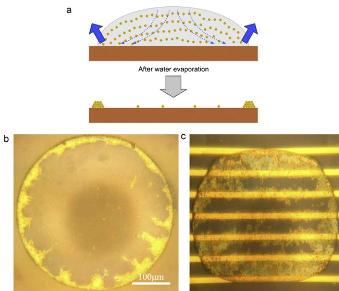
**Fig. 1.** Optical images of printed nanoparticle films: (a) schematic view of the self assembly of gold nanoparticles after water evaporation; (b) 1000 drops of 100 nm gold nanoparticles deposited on oxidized silicon substrate; (c) 1000 drops of 100 nm gold nanoparticles deposited on gold electrodes fabricated on top of oxidized silicon substrate.
