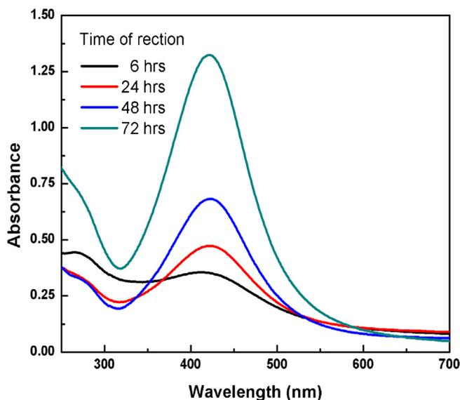
Fig. 2. UV–vis spectra recorded as a function of reaction time for Ag NPs synthesized using 1 mM  $\text{AgNO}_3$  and 0.1% LBG solution at  $60^\circ\text{C}$ .
