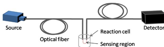
Fig. 1. Experimental set up for optical fiber based sensor for detection of hydrogen peroxide.
