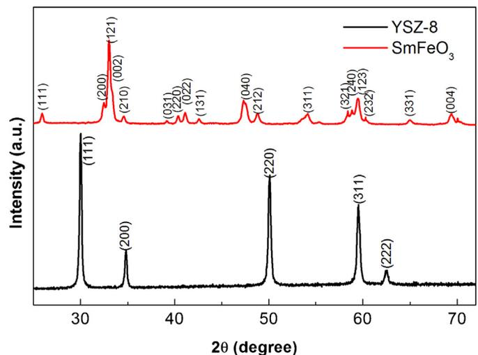
Fig. 2. X-ray diffraction patterns of the synthesized powders YSZ-8 and  $\text{SmFeO}_3$ .
