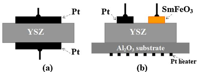
Fig. 1. Schematics of the cell Pt/YSZ-8/Pt (a) and the sensor Pt/YSZ-8/ $\text{SmFeO}_3$  (b).
