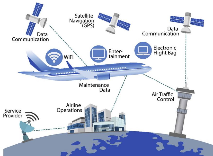
Fig. 1. Visualization of interlinked systems in the civil aviation domain showing several potential vectors for cyber-attacks. The figure is based on Vereinigung Cockpit (2017).
