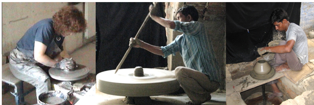
Fig. 1. Wheels used in the three cultural settings. From left to right: the electrical (pedal operated) wheel used by the French potters, the high inertia stick-wheel used by the Prajapati potters, and the low-inertia kick-wheel used by the Multani potters.
