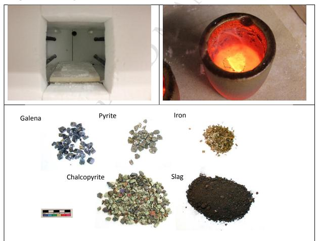
Figure 1 Experiment set-up. Left: furnace chamber used in this experiment. Right: crucible retrieved from furnace after reaction. Bottom: Raw materials used in these experiments.
