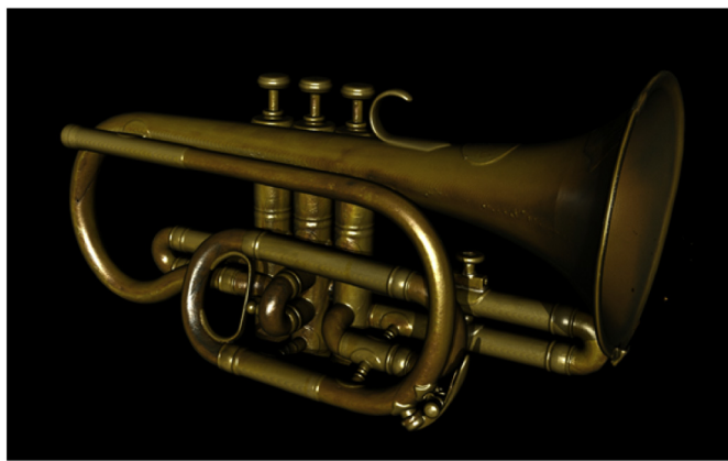
Fig. 1. Outer view of the tomography study of a 19th century cornet with thermal neutrons at the NEUTRA facility at PSI; the voxel size is on the order of 0.1 mm.
