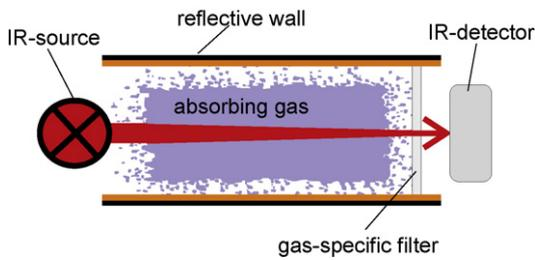
**Fig. 1.** Sketch of a common NDIR gas sensor with its basic building blocks: IR-source, optical path containing the sampling gas, filter, and IR-detector.
