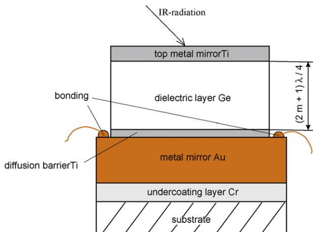
**Fig. 2.** Sketch of the implemented Fabry–Perot structure (dimensions not to scale). The thickness of the germanium layer corresponds to the infrared absorption wavelength required for the CO<sub>2</sub> detection.
