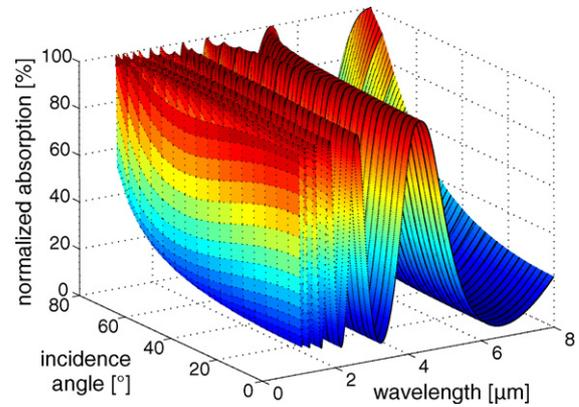
**Fig. 3.** Simulated absorption of a bolometer assembled similar to Fig. 2. The absorption depends on the IR-wavelength and the incidence angle of the IR-radiation.
