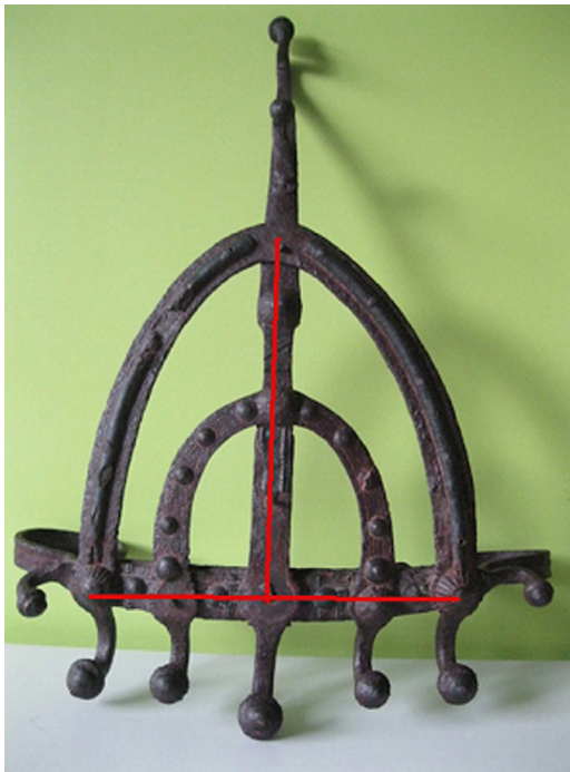
Fig. 1. The Qibla Finder. Red lines are projections of Equator (0°), Tropic (23.5°), Polar Circle (66.5°) and Pole (90°). The distance on the tool of Pole from Equator is 200 mm and corresponds to the radius of a local sphere. The two branches of the larger ogive are the planar projection of the -30^\circ and +30^\circ meridians. In the inset the detail of a fine scale spanning 15^\circ . Base hooks are at a distance of 15^\circ . All measurements reported in the figures where the Qibla Finder is used may be easily checked by the reader scaling a digitalized image in which the reference points are the extremes of the with line and their distance is 200 mm.
