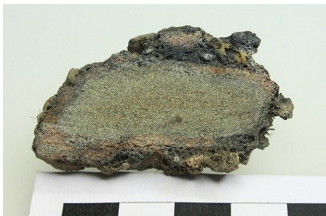
Fig. 1. A photograph of a vitrified sample from the wall at the Wincobank site, Yorkshire, U.K. (reproduced with permission from Hearne, 2015). The scale bar at the base of the sample is divided into centimetres.
