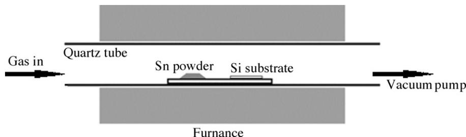
Fig. 1. Experimental setup. Tin powder and the silicon substrate were separated by 10 mm in the center of the quartz tube.
