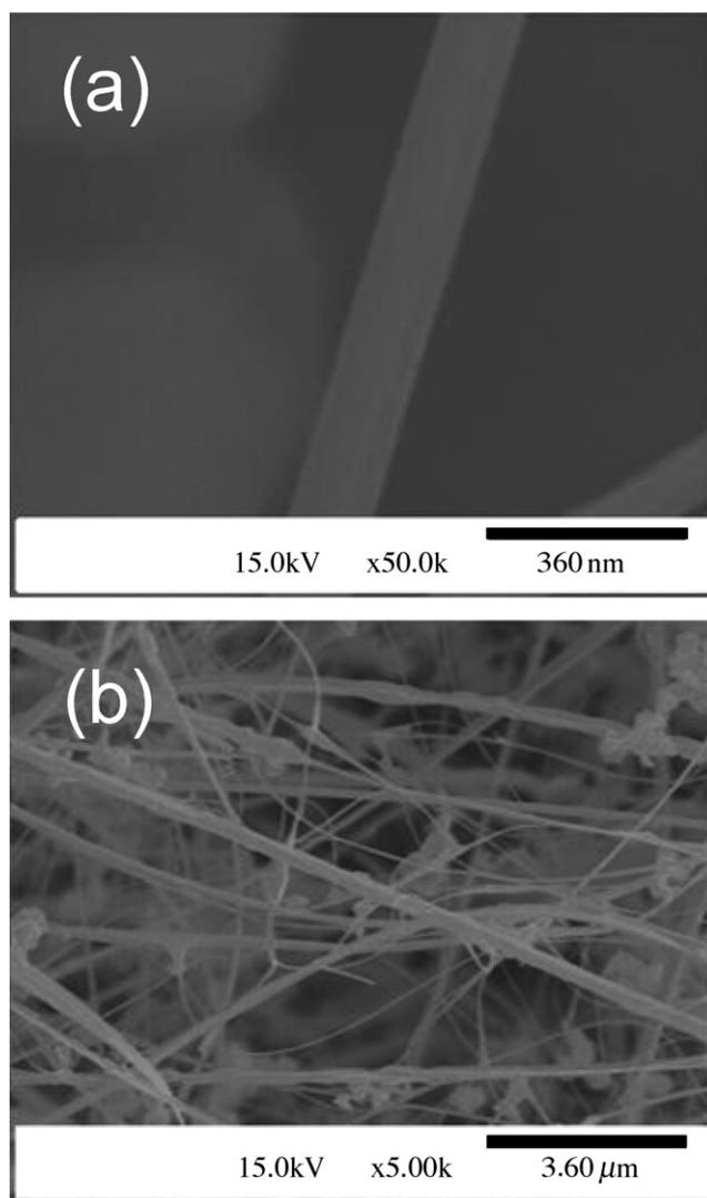
Fig. 2. The SEM images of SnO<sub>2</sub> nanowires synthesized at 800 °C on a Si (1 1 1) substrate.
