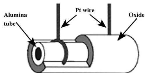
Fig. 1. The photography of gas sensor.
