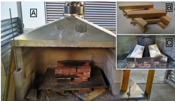
Fig. 1. (A) Cookstove testing chamber with a traditional Peruvian brick channel stove resting atop a metal plate. The hood vented to a chimney augmented by a fan that can be seen directly above the apex of the hood. (B) The wood was arranged in a 'log-cabin' configuration made of sticks measuring 2 cm \times 2 cm \times 13 cm. There were 4 layers of sticks, with each layer containing 2 sticks. (C) Skirt surrounding pot.
