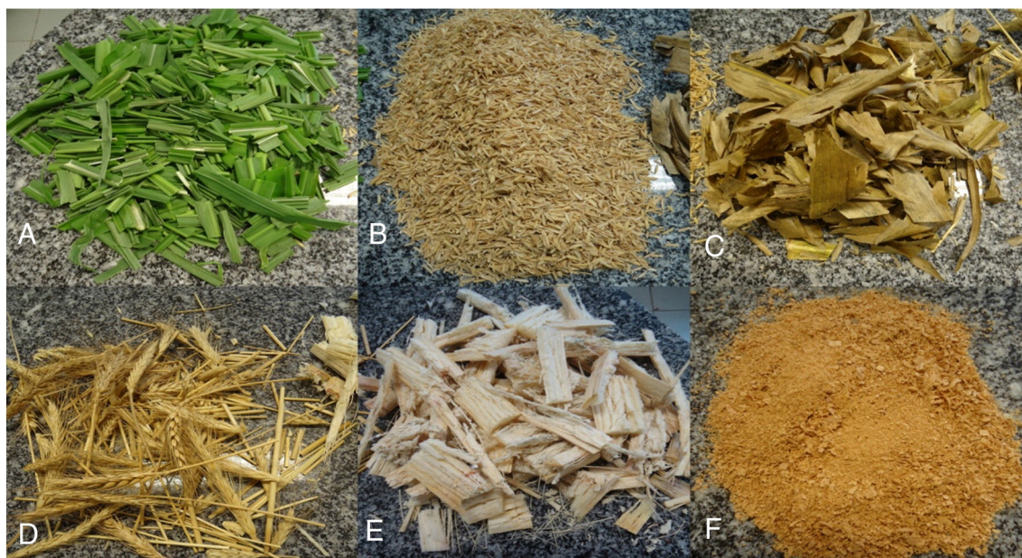
Fig. 1. Samples of the biomass analyzed in this work. a) Elephant grass, b) rice husks, c) corn straw, d) wheat straw, e) sugarcane bagasse, and f) wood chips.
