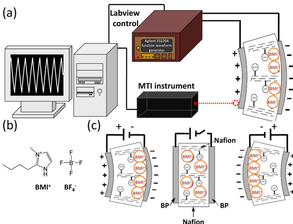
**Fig. 1.** (a) Schematic of the BP/BMI<sup>+</sup>-Nafion/BP composite actuator and actuation measurement setup using an MTI laser displacement sensor; (b) molecular structure of BMI<sup>+</sup>BF<sub>4</sub><sup>-</sup>; (c) actuation mechanism of BP/BMI<sup>+</sup>-Nafion/BP composite actuator.
