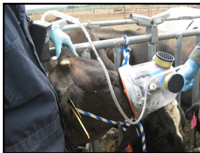
Fig. 1. Photo illustrating the system employed for breath sample collection in the cattle. Inspired air first passes into the mask through three charcoal filters and one-way valves to remove environmental VOCs. Expired air passes out of the mask through two one-way valves and through the tubing inserted into a hole in the front of the mask. Air in the tubing passes through a glass cartridge containing sorbent material (Tenax™) and is exhausted through the hand-held suction pump.
