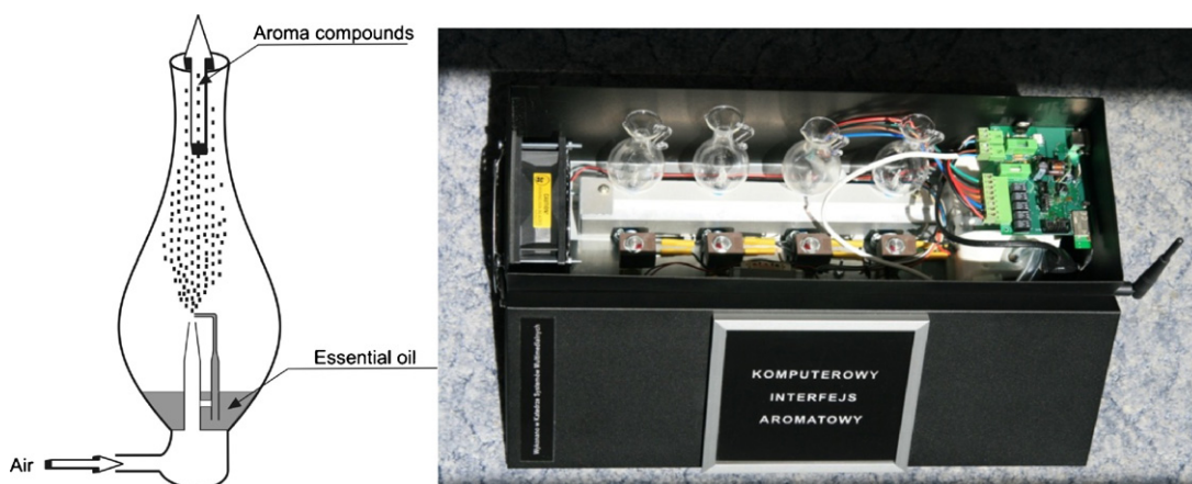
Fig. 1. Nebulizer for oil essential scents emission powered by compressed air (left) and the prepared prototype device (right) that can emit four different aromas.
