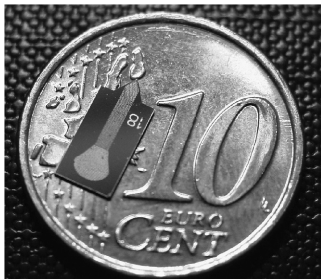
Fig. 2. A \mu PESI chip on a 10 euro cent coin.
