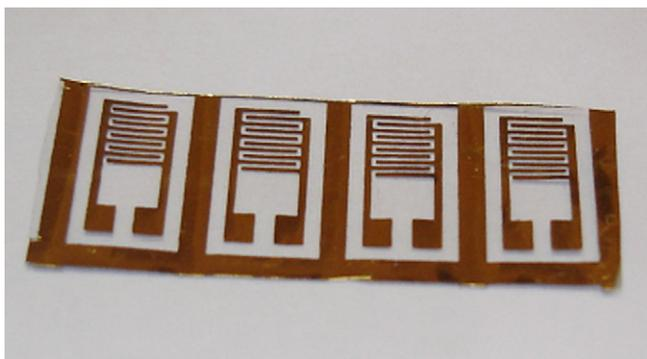
Fig. 1. The photo of the humidity sensors on a PET substrate.
