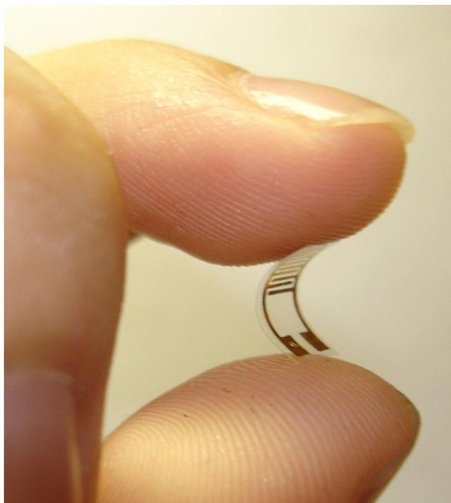
Fig. 2. The photo of a flexible humidity sensor.
