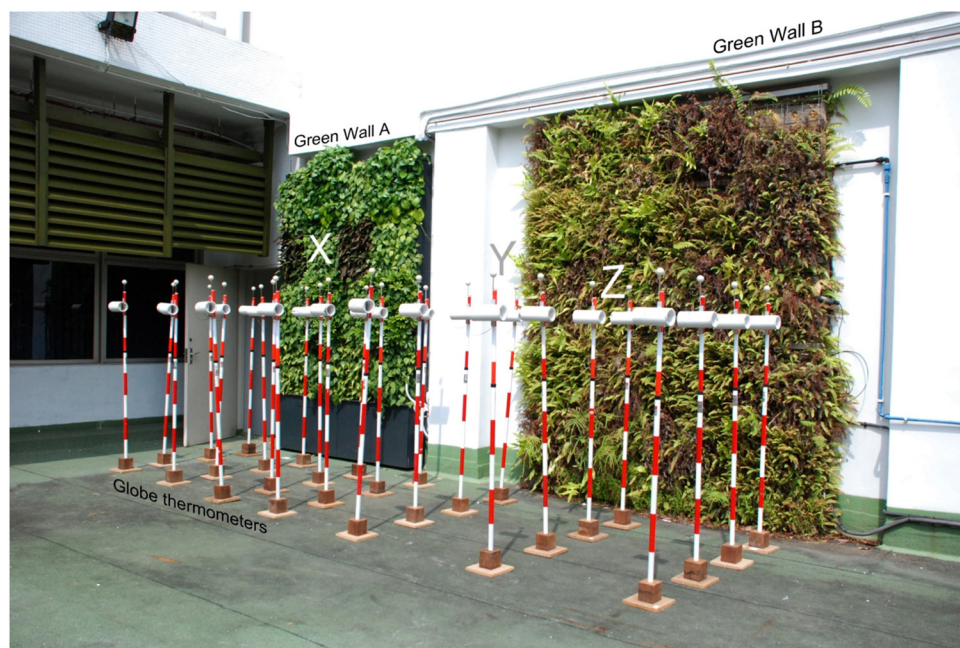
Fig. 2. Measurement setup. Globe thermometers were attached to poles with white PVC pipes housing surface and air temperature loggers.
