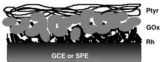
Scheme 1. Schematic representation of the biosensors.
