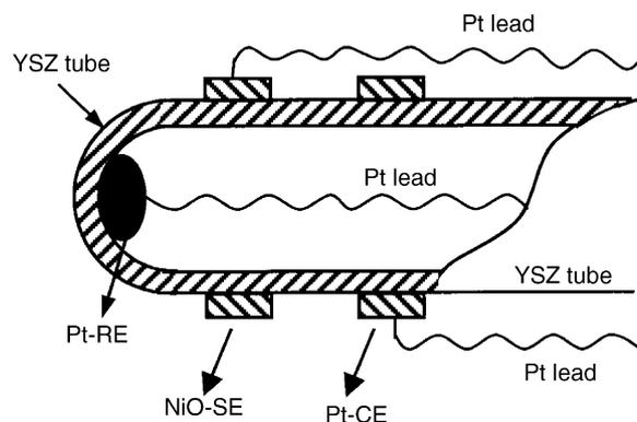
Fig. 1. Schematic cross-sectional view of NO<sub>2</sub> sensor using YSZ tube and NiO-SE.
