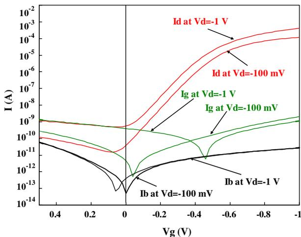
Fig. 3.  $I_d$ - $V_g$ ,  $I_b$ - $V_g$  and  $I_g$ - $V_g$  at  $V_{ds} = -100$  mV and  $-1$  V characteristics of pMOSFET whose body is grounded ( $W/L = 2.5 \mu\text{m}/0.11 \mu\text{m}$ ).
