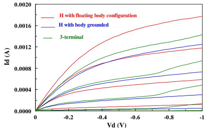
Fig. 5.  $I_d$ - $V_d$  comparison of H-gate with either body grounded or floating-body configuration and 3-terminal pMOSFET with  $V_g$  from  $0$  to  $-1$  V by  $0.2$  V steps ( $W/L = 5 \mu\text{m}/0.11 \mu\text{m}$ ).
