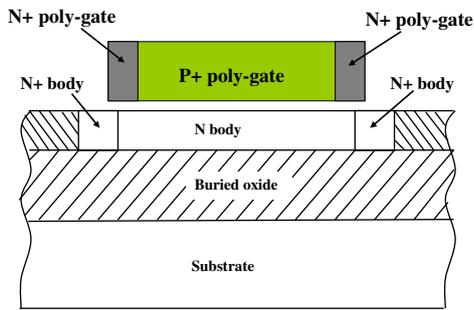
Fig. 2. Cross-sectional view taken from line A–A of Fig. 1, illustrating H-gate PD SOI pMOSFETs with p+ poly-gate, partial n+ poly-gate and n type substrate.
