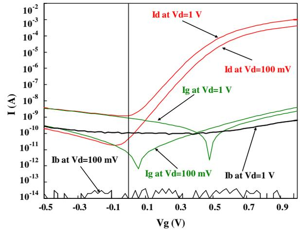
Fig. 4.  $I_d$ - $V_g$ ,  $I_b$ - $V_g$  and  $I_g$ - $V_g$  at  $V_{ds} = 100$  mV and  $1$  V characteristics of nMOSFET whose body is grounded ( $W/L = 2.5 \mu\text{m}/0.11 \mu\text{m}$ ).
