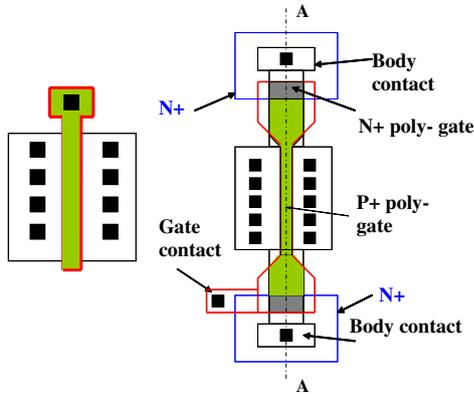
Fig. 1. Top view layouts of 3-terminal (left) and H-gate PD SOI pMOSFETs with two body contacts (right).
