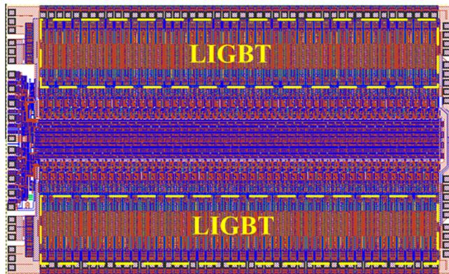
Fig. 2. The layout of plasma display panel (PDP) scan driver IC.
