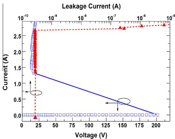
Fig. 3. Measured TLP  $I-V$  characteristic of SOI LIGBT.
