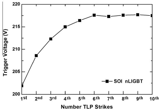
Fig. 5. Trigger voltage evolution as a function of the TLP zapping time.
