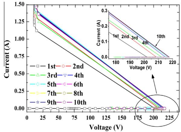
Fig. 4. Measured  $I-V$  curves of SOI LIGBT subject to repetitive TLP stresses.
