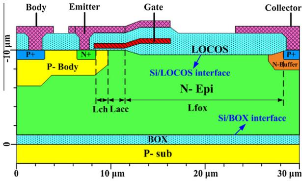
Fig. 1. Cross-section of the investigated LIGBT structure.
