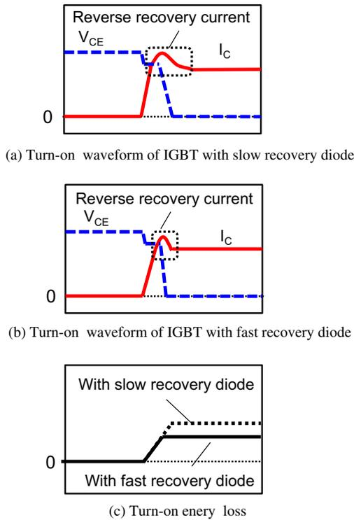
**Fig. 1.** Image of reduced turn-on energy with fast recovery diode. (a) Turn-on waveform of IGBT with slow recovery diode. (b) Turn-on waveform of IGBT with fast recovery diode. (c) Turn-on energy loss.
