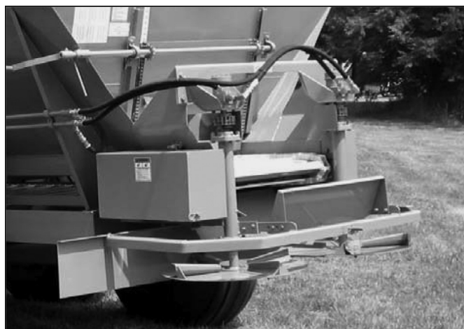
Fig. 1. Close up of dual-plate horizontal spinners and conveyor delivery system.
