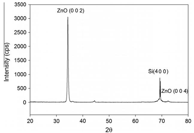
Fig. 2. HR-XRD of RF-sputtered ZnO thin films on thermally oxidized n-Si (100).
