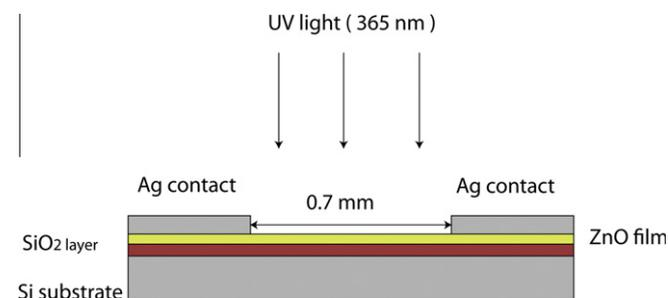
Fig. 1. Cross-section diagram of the ZnO MSM photodetector.
