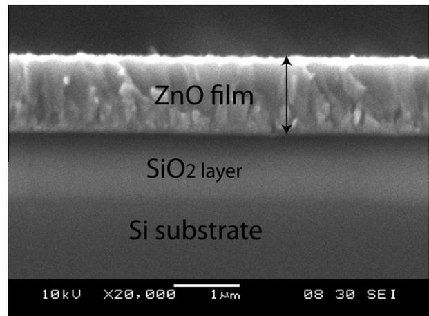
Fig. 3. SEM cross-section image of the prepared ZnO films. The bar length is 1  $\mu\text{m}$ .
