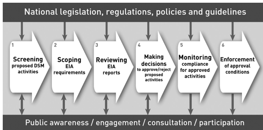
Fig. 1. The regulatory steps of the EIA process, including input and direction from legal and policy instruments and the public.
