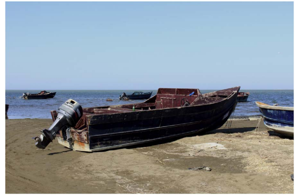
Fig. 1. Self-manufactured boat, so-called bayda is the small open motor boat between 3 and 11 m in length powered by outboard engine up to 1000 hp.
