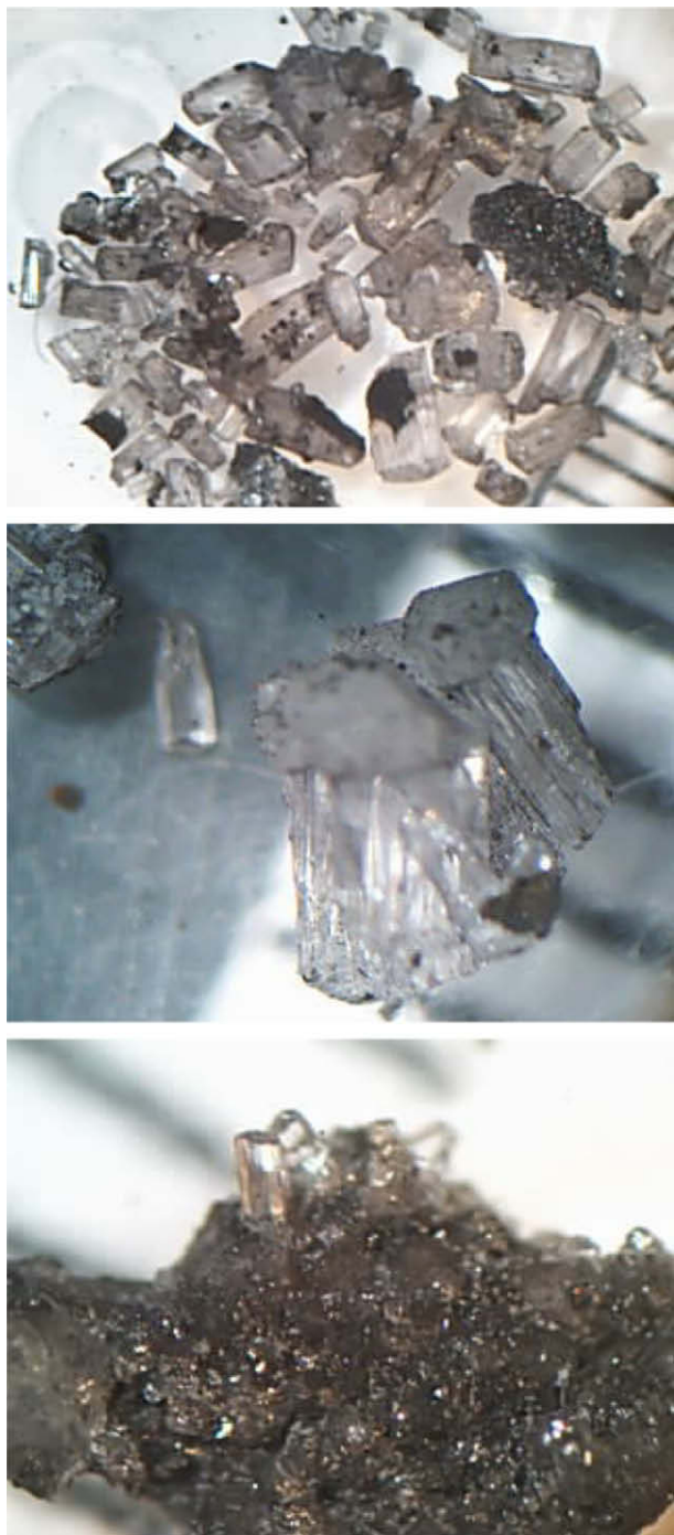
Fig. 1. Top: selection of CAN crystals. Middle: CAN crystals growing on well faceted SOD crystals. Bottom: di-hexagonal CAN crystals on a raft of SOD and magnetite (scale = 1 mm divisions).
