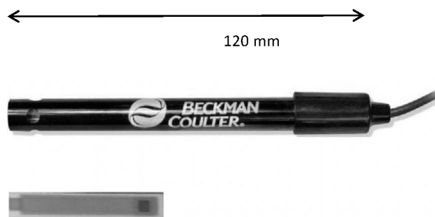
Fig. 1. Comparison of commercial liquid-filled (top) and screen-printed (bottom) reference electrodes, shown on same scale. The thick-film device shown is less than two times smaller in length and only a couple of millimetres thick, but can be miniaturised much further to only a few millimetres square if desired.
