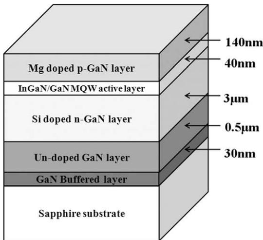
Fig. 1. A schematic diagram of GaN based green LED substrate.
