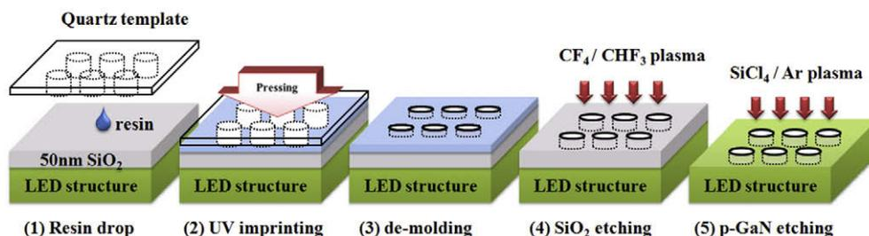
Fig. 2. Schematic illustration of overall processes flow for patterning of p-GaN top cladding layer of LED using nanoimprint lithography.
