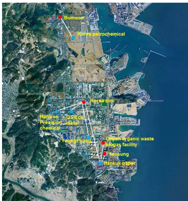
Fig. 1. Status of the energy IS at the Onsan national industrial park in Ulsan (red: heat source, blue: heat sink).
