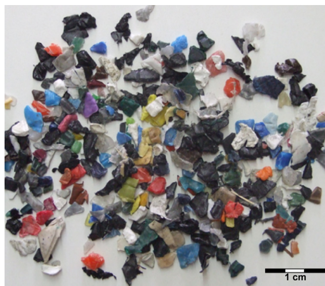
Fig. 1. Source sample of polyolefins from building and construction waste.
