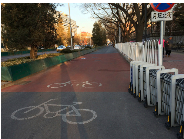
Fig. 1. Physical fence for segregating cars and bikes in Beijing.
