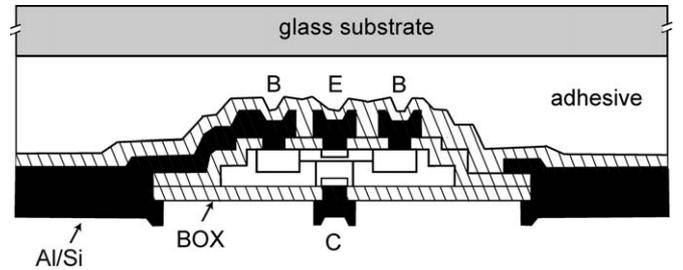
Fig. 1. Schematic cross section of a silicon-on-glass NPN bipolar transistor.
