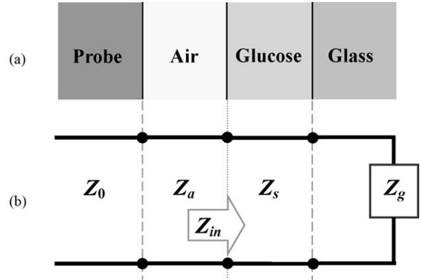
Fig. 2. Schematic diagram of (a) probe-sample and (b) its equivalent model.
