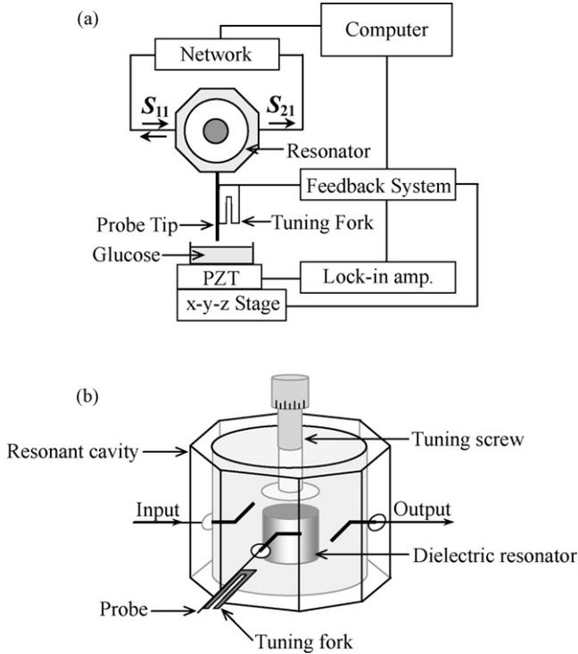
Fig. 1. (a) Block diagram of NFMM with tuning fork distance control and (b) NFMM microwave resonator and probe tip assembly.
