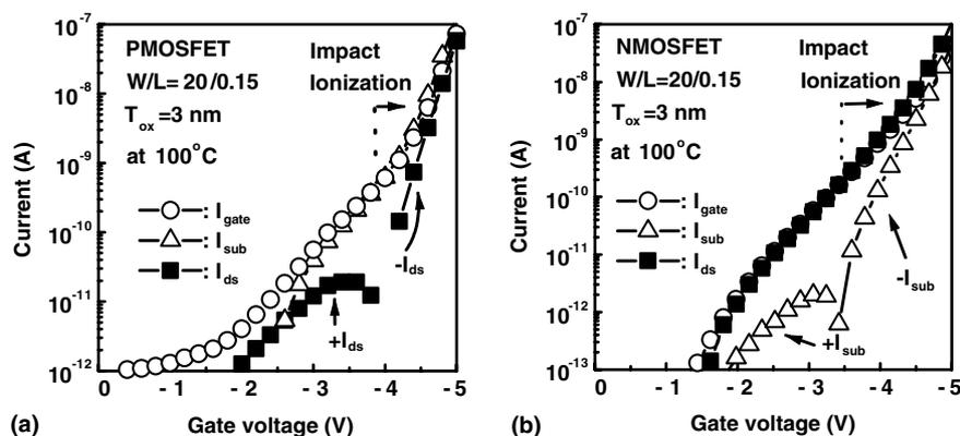
Fig. 1. Carrier separation  $I$ - $V$  curves for 3 nm-thick gate oxide devices ( $W/L$ : 20  $\mu\text{m}/0.15$   $\mu\text{m}$ ) measured in negative bias: (a) p-MOSFET; (b) n-MOSFET.
